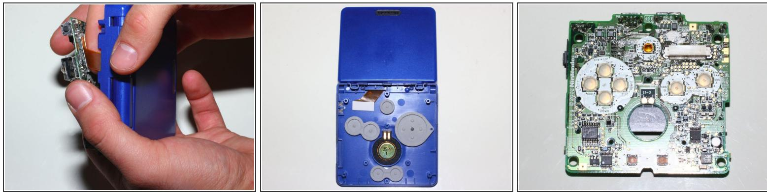
**⚠** Carefully using fingers, detatch display ribbon from its socket. This ribbon is especially hard to remove due to the angle in which you'll need to remove it.
